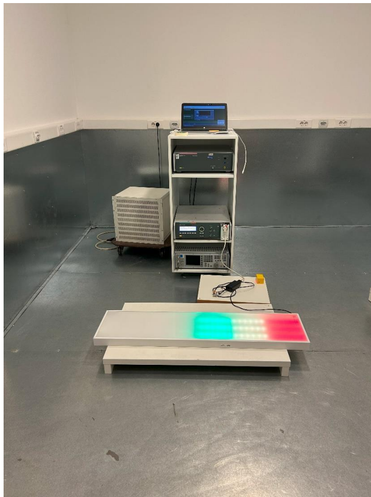
Figure 28: Electrical fast transient/burst and Surges immunity measurement
